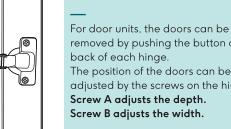
removed by pushing the button at the The position of the doors can be adjusted by the screws on the hinges.
