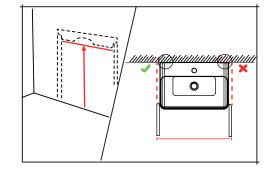
Mark the location of both mounting plates, ensuring that they are positioned inside the unit's side panels. Note the opening width of door units. Make sure that there are no hidden pipes or cables in the wall. The fixings supplied are for solid walls. For hollow or stud walls use specialist fixings.
