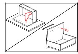
The front panel can be adjusted by the screws located at the sides of the
